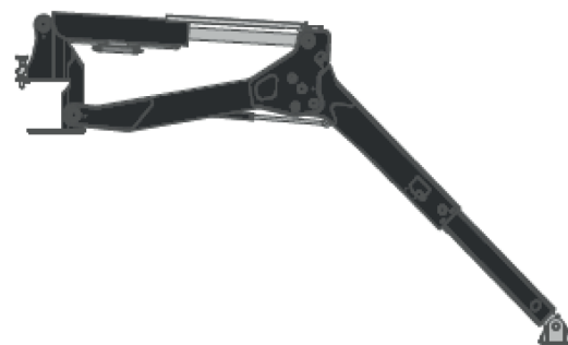
45° EXTENSION WITH OUTRIGGER COMPLETELY EXTENDED
